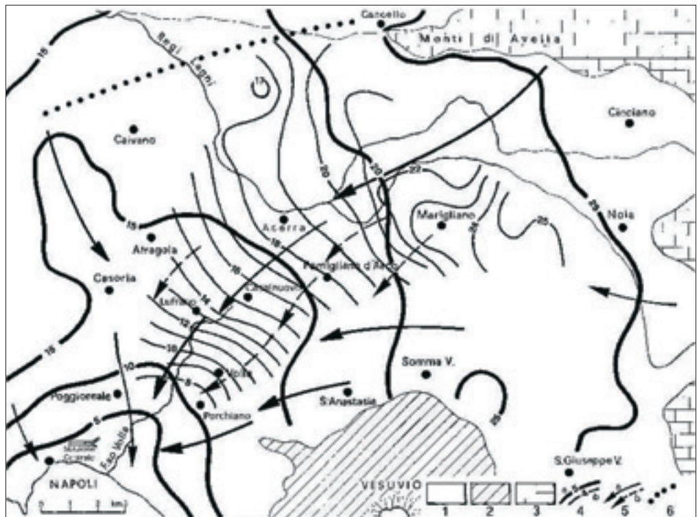
Figure 13 – Water table morphology of the eastern of Naples in October-November 2002 (Autorità di Bacino Nord Occidentale della Campania, 2004, modified and integrated). Legend: 1) Pyroclastic-alluvial deposits; 2) Lavas and pyroclastic deposits; 3) Carbonatic rocks; 4) Piezometric contour lines (m a.l.m.): a) semiconfined aquifer; b) unconfined aquifer; 5) Direction of groundwater flow: a) semiconfined aquifer; b) unconfined aquifer; 6) Groundwater divide.
